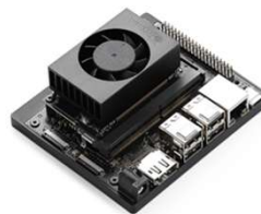
Edge device example for AI vision deployment (NVIDIA Jetson Orin Nano)
